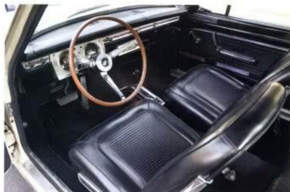
Optional simulated woodgrain steering wheel stands out against standard interior; all Barracudas featured vinyl-clad front buckets—reproduction material is available.
