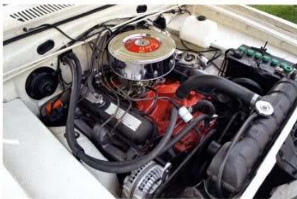
Every engine offered in the Barracuda is rebuildable, including this 235hp V-8; lack of fan shroud indicates this car was not equipped with optional air conditioning.
