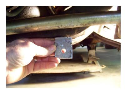
Here is a mock up of the given directions for the swaybar. I feel even if you weld the angle bracket to the K frame the stress on the bolts would bend and snap them. Also the pivots are too close to the center of the bar.
