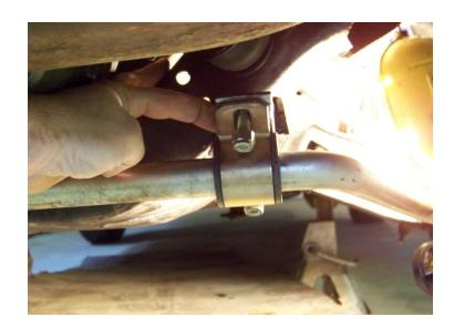
Here you get a better idea of how it will look. The mount will be angled a bit and welded to the angle piece and that new asembly will get welded to the K frame.
