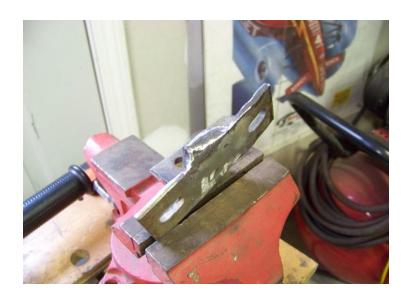
Tack weld the mount to the K frame and double check your measurements now. If they are good then complete the welds an grind them to check for defects.
