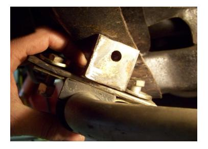
Take some measurements and mark your K frame. Then you can hold the pieces together for tack welding.
