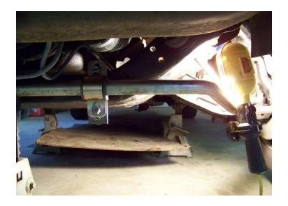
Here is where I will mount the brackets using the hardware given in the kit. notice how far out the pivot is giving the bar better support.
