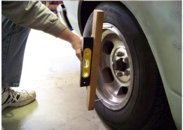
**Put the car on the floor and bounce the front end a few times to settle it. Re check the level, if it's off one way or the other, jack the car up and adjust as necessary.**
