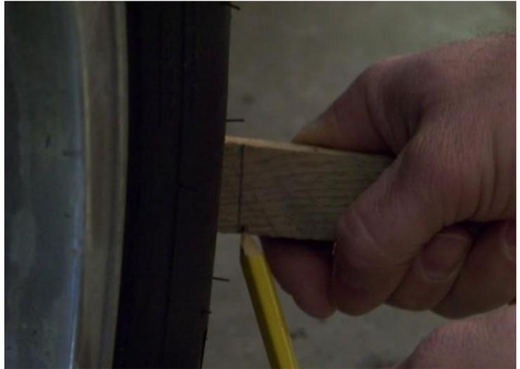
**If the line for the “front” is closer to the screw than the line for the “back” then you have tow in, if its reversed you have tow out.**
