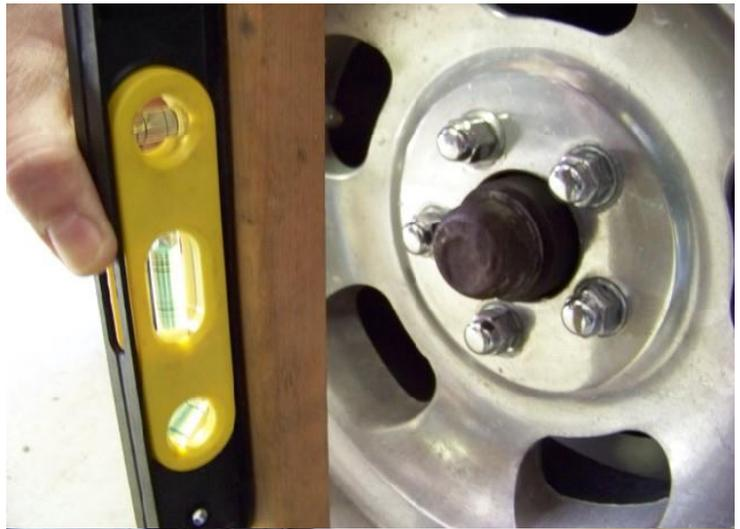
**Next is the Tow. The one thing we are not going to worry about is if the steering wheel is straight. The alignment shop will get that right. Hold the Tow tool with the screw up against outside of the front RF tire. (Have someone help hold it on that side if you need to.)**
