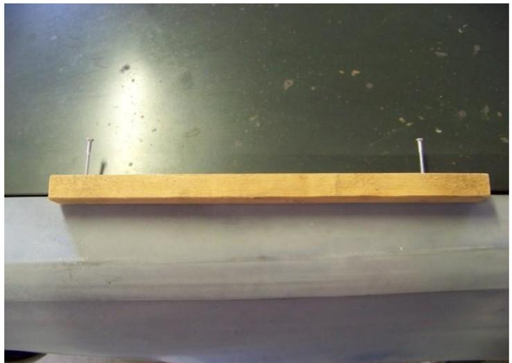
**For our Tow tool a long piece of wood trim or two long ones mounted together and one 3 inch wood screw. As you can see from my tool I chose to duct tape the two pieces together.**
