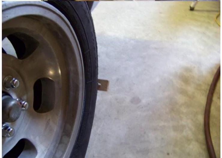
**With the pencil held against the outside of LF tire, mark the tool. Mark this line "front" or "f".**
