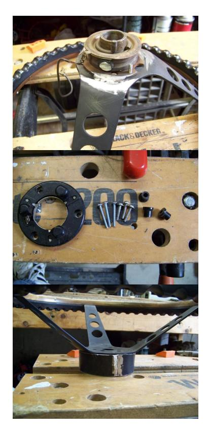
Notches were cut in the ring and the third spoke cut off the wheel. The ring was test fit and trimmed many times to insure a good even fit.
