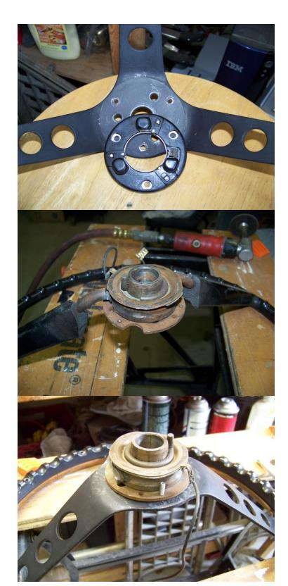
... it was welded in place. If you don't have a welder, or don't trust your welding skills, have a professional do this. The consequences of a failed weld here could be devastating.
