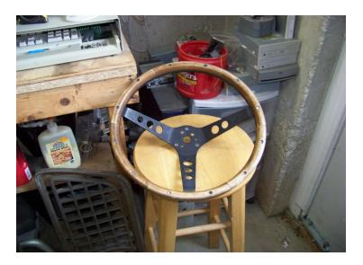
Using the horn ring as a guide, I centered it, marked and drilled holes so the bolts that mount the ring and horn button can pass through the wheel and mount the hub that I will use from a un-restorable original.
