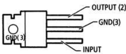
Now you need to make the electrical connections. There are three pins that come from the chip. In the pictures, the input is the lowest pin, the ground is in the middle, and the output is at the top. First, bend the middle pin upwards slightly. Then, angle the input pin towards the "I"
