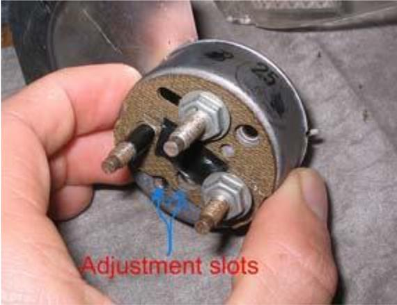
There are a couple of slots you can see in the back of the gauge that also give you a little adjustment. The lower one moves the pivot point of the needle with respect to the bimetallic arm. The upper one shifts the whole thing right or left. Not a lot of adjustment in either case, but if you're just a little off one way or the other it can help. It's also hard to make either adjustment a slight one. They tend to be sticky.
