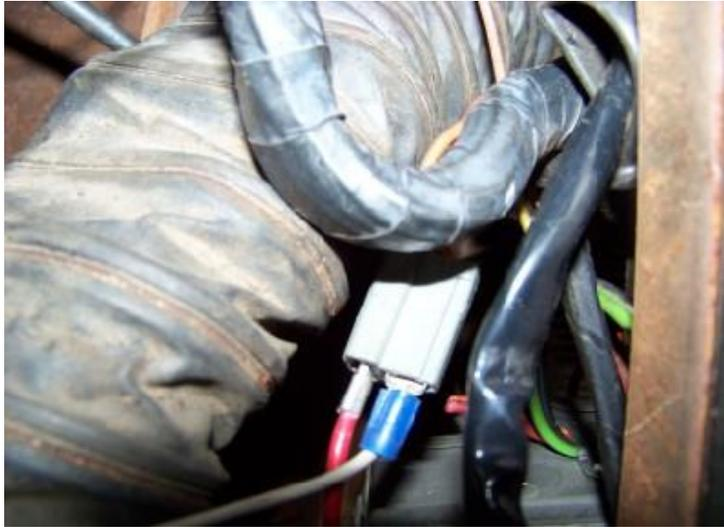
**You can buy a buzzer or chime from your local auto parts store or electronics supply house. Just ground the chime and connect the power lead to the 87A pole on the relay.**
