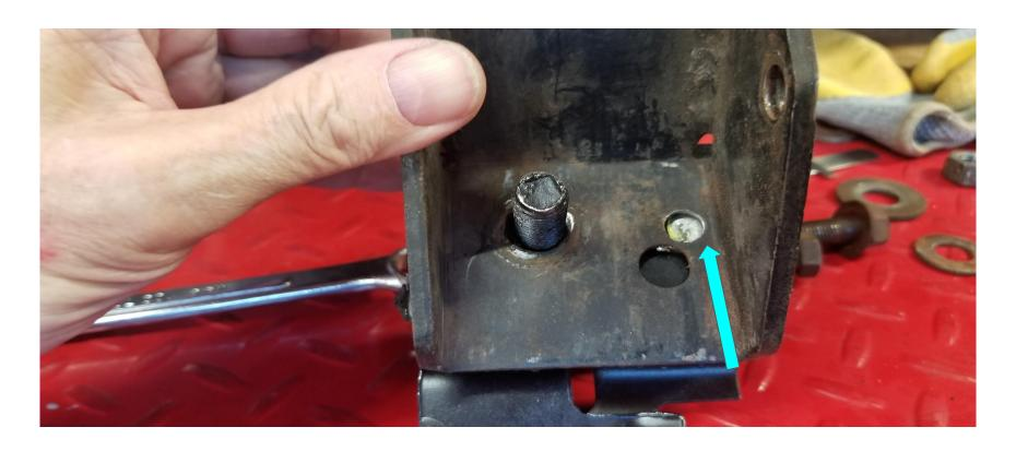
This is the 2469 model. I installed it first, but it was too soft and too short. It dropped the engine down enough that the headers interfered with the steering coupler and the driver's torsion bar!
