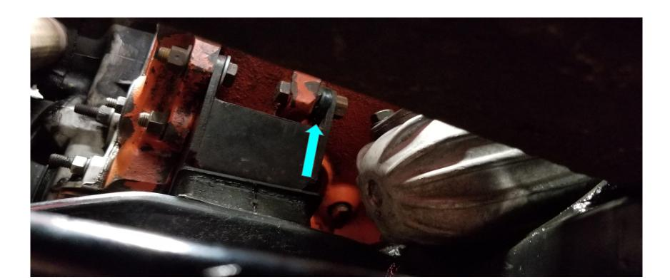
Finally installed and tested! In the end, it's simply a matter of drilling a new alignment hole in the mount perch - and the regular skinned knuckles trying to reassemble the bits. (I found it easiest to attach the perch to the top of the motor mount on the workbench, and then install the assembly.)
