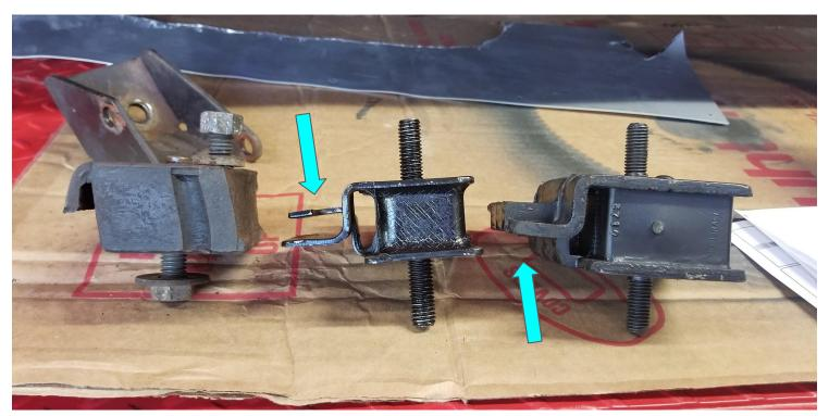
This is a different view showing the bottom of the three mounts. Note that the middle one has an extra 'button' that should have a corresponding alignment hole, but the k-member doesn't have that hole. This is another point in favor of the 2710 model on the right.
