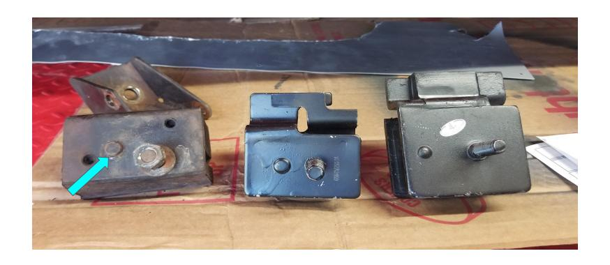
This is the driver's motor mount perch, as seen from inside the engine. (!) Note the new hole on the right side that matches the button on the top of the 2710 mount.
