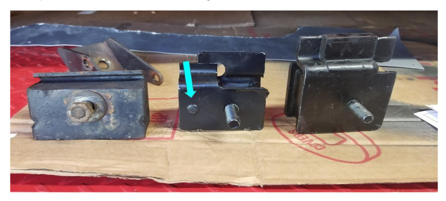
Here is a view of the top of the mounts. Note that the original one had a button diagonal from the bolt; there is a matching hole in the motor mount perch.
