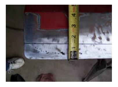
Using my 4 1/2 inch angle grinder with a cutting disc I carefully cut through the outer sheet metal along the marked line. Be careful not to cut too deep on the edges.
