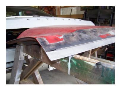
You can see how I cut the ends to fit under the existing trunk metal. I'll need to do a little extra welding to close the gap here. The corners will need to be welded and ground to get the radius correct. That won't be too difficult.
