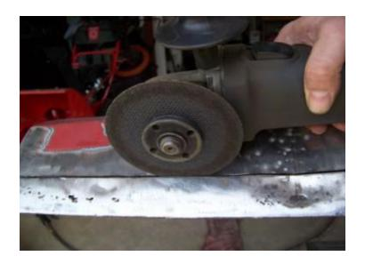
When you are done with the cutting, the upper and lower sections will spread apart.
