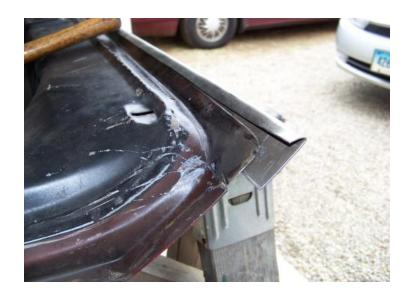
With the lip done it's time for the corners. Using the angle grinder I cut a arched line to the top corner of the bent lip and then cut the remaining excess lip off, leaving a flat flap to peen over on the end.
