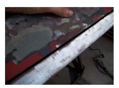
Using a small pry bar start to pry the inner lip up and away. Take your time and do not force it. There are spot welds that will need attention and we do not want to damage the inner trunk lid.
