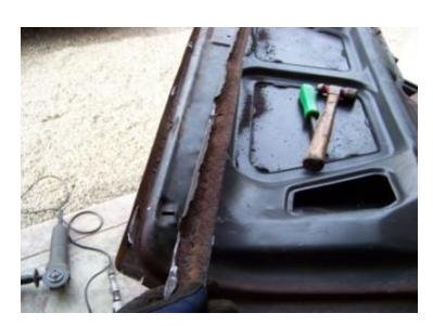
Clean up the sheet metal with a file to remove any loose metal. Now would be a good time to blow out any debris or rust floating around inside the lid.
