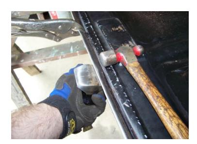
Once you get it close to closed, push one of the ends in tight to the trunk lip, clamp it down and continue to hammer and dolly the edge flatter and flatter.
