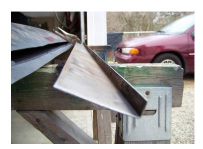
I started by putting a flange on the top edge of the new patch so it fits under the the existing sheet metal on the trunk. This will allow us to weld the seam without blowing through and making the final body work a little easier for the novice.
