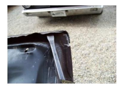
And the lip is off. Don't toss the lip yet. We will need it as a template for the new sheet metal. Take this time to grind off any left over metal around the spot welds and clean up both sides of the inner lip with a wire wheel.
