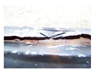
...Then carefully grind the edge until you break through and can see the two separate parts. This will make it easier to pry the lip up around the welds.
