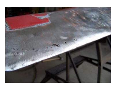
I measured up an inch and a half and marked the lid all the way across as a guide line for the grinder.
