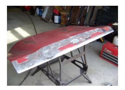
Here you can see the rust. Its worse on this end but there is rust on the right corner too. You can see the old damage I will repair later.
