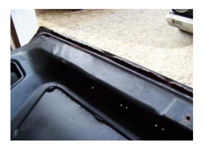
Using the grinder cut around the weld like this to relieve the stress on the lip...
