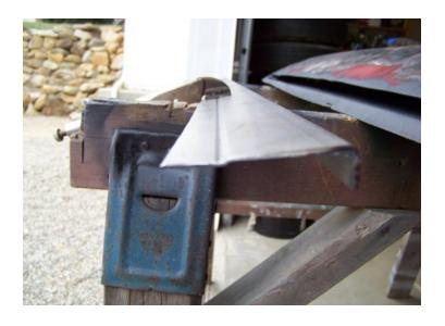
Get the hammer out, we need to bend the seam over to start the fitting to the edge of the trunk. Don't go too far, just enough to get it at a 45 degree angle.
