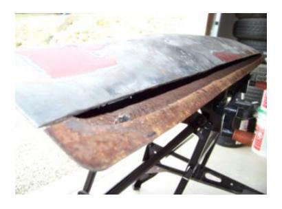
I took the extra step of treating the bare rust with a spray rust converter. I did both sides of the inner lip and I sprayed as far inside the trunk as I could. Wait until it's dry and add a second coat. You do not want to do this repair again and now is the time to protect the metal. Other treatments like Por15 can be used as well.
