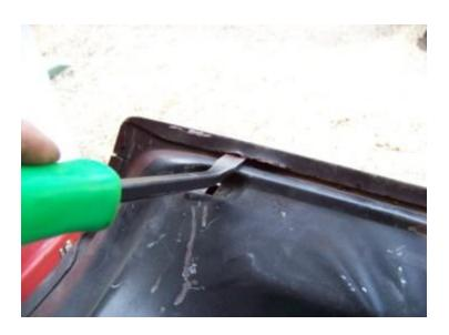
When it looks like this stop and address the spot welds. You can see the sections that are still stuck and need work.
